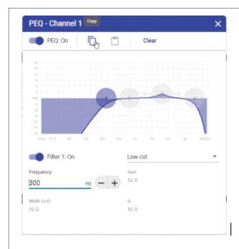
Fig. 6 To tailor your filters within the PEQ, choose the type of filter and adjust the settings as needed. Once you have it as you like you can copy it to other channels.
